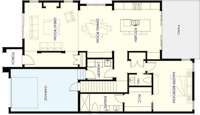
○ Main Floor Plan Floor Area = 1398 sq. ft. (Not including Garage)
